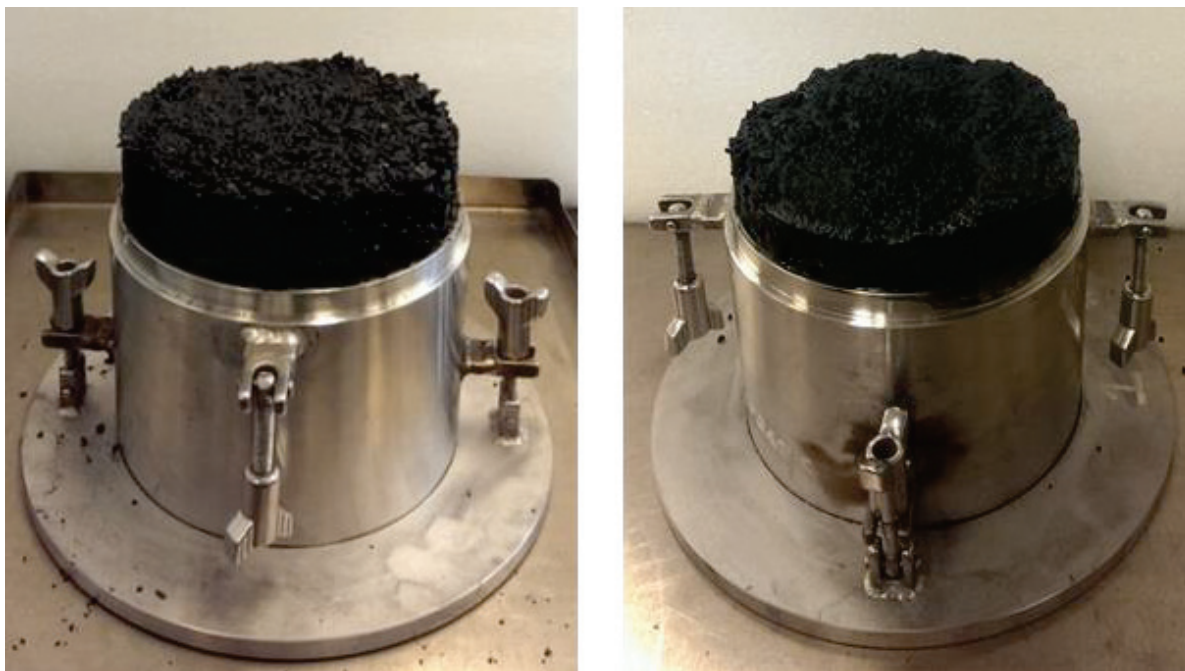
Figure 1.5.5.3.4.1 – Photographs showing valid tests for a partially saturated test portion (left) and a near fully saturated test portion (right)
