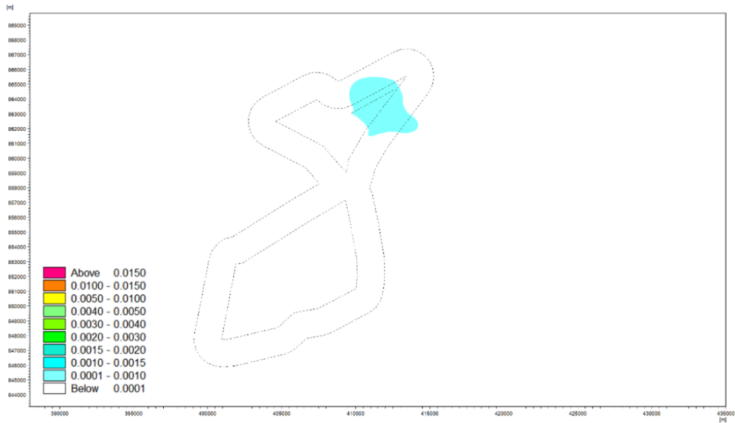
Figure 5.32. The sediment layer thickness distribution [m] after completion of works conducted in the technology of water jetting with the device moving at a speed of 200 \text{ m}\cdot\text{h}^{-1} in the area of laying the inter-array cable lines in the Baltica-1 OWF field in cohesive soil
