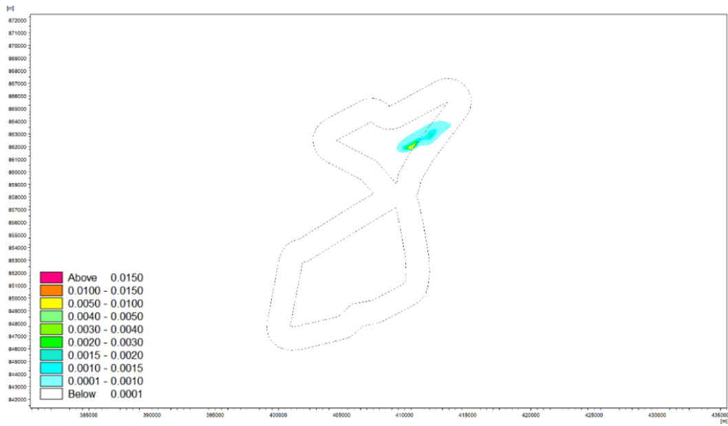
Figure 5.6. The distributions of sediment layer thickness [m] after the completion of the preparation of the substrate for the installation of a Ø 55 m gravity-based structure in cohesive soil, in the Baltica-1 OWF field
