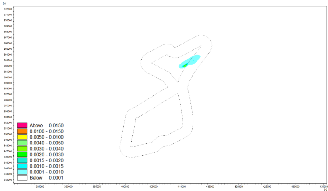
Figure 5.11. The distributions of sediment layer thickness [m] after the completion of the preparation of the substrate for the installation of a Ø 55 m gravity-based structure in non-cohesive soil, in the Baltica-1 OWF field
