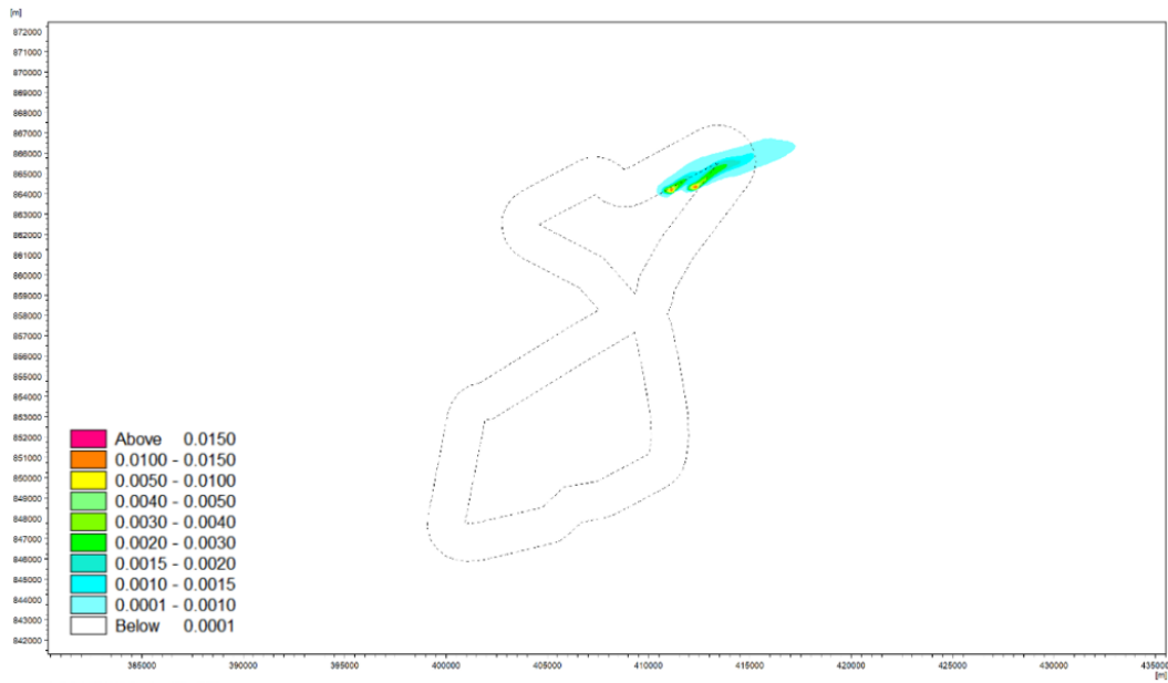
Figure 5.52. The distributions of sediment layer thickness [m] after the completion of the seabed substrate preparation for the installation of \varnothing 55 m gravity-based structures in two locations simultaneously (in cohesive soil), in the Baltica-1 OWF field
