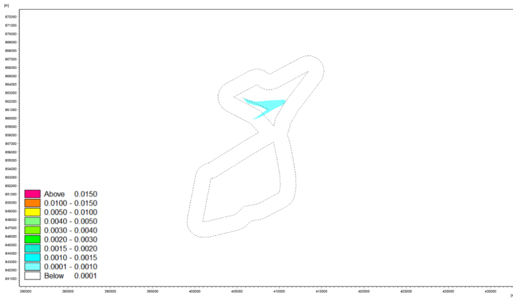
Figure 5.47. The sediment layer thickness distribution [m] after the completion of works conducted in the technology of ploughing with a device moving at a speed of 200 \text{ m}\cdot\text{h}^{-1} over the area of the inter-array cable line laying in the Baltica-1 OWF field in non-cohesive soil
