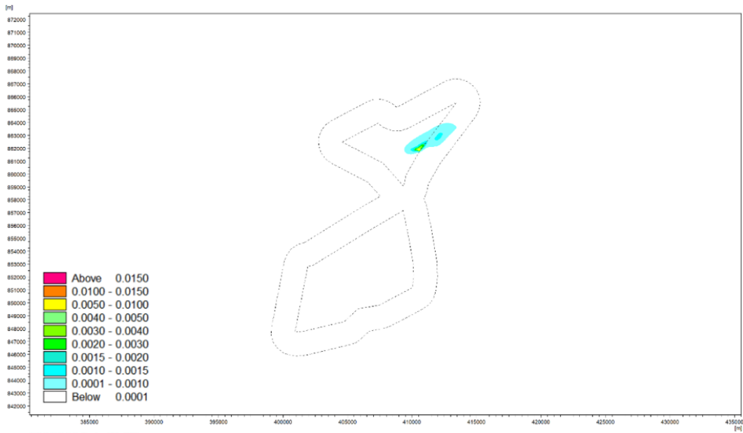
Figure 5.16. The distributions of sediment layer thickness [m] after the completion of the preparation of the substrate for the installation of a Ø 45 m gravity-based structure in cohesive soil, in the Baltica-1 OWF field
