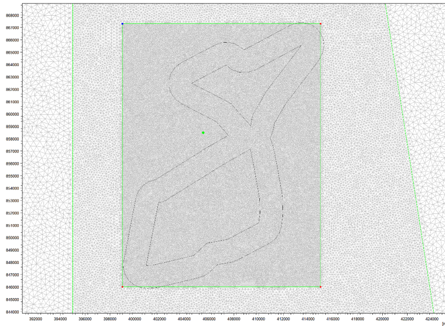
Figure 3.1. The location of the calculation model, including the assumed dense numerical grid, against the Baltica-1 OWF area
